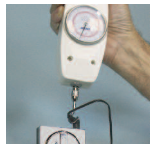
Wire Pull-out Test
